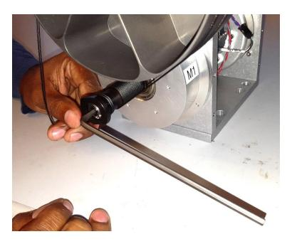
9. Using the 23mm open end wrench and the torque wrench, tension the one-way tension clutch to 22.5 in-lb or 26 kg-cm.
