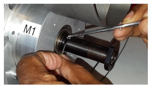
4. Rotate Pinion 1 so the cable begins to spool. Overlap the cable on top of the outer termination in the anchor like shown.
